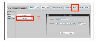
7. Either hit the **Tune** button or under the Start menu, hit Tune then **ProTune**. Select the Nucleus you wish to tune to. For routine experiments, you can use **Coarse** Quality, as this is fastest. If you are running a proton-decoupled phosphorus, carbon, or other heteronuclear experiment, make sure to tune the heteronucleus first and also tune proton! e.g. for 31P{1H}, tune P31 and then H1.
